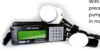
With data quality exceeding standard proton precession and comparable to costlier optically pumped cesium units, the GSM-19 is a standard in many fields, including:
