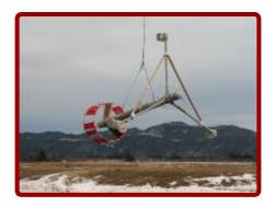
As the core of GEM's airborne solutions, the GSMP-35A has improved its sensitivity to 0.0003 nT @ 1Hz (previously 0.0005), making it the highest sensitivity potassium magnetometer in the world. The sensitivity is the highest in all weather conditions, which enables enhanced resolution of geological and cultural features in a variety of applications.
